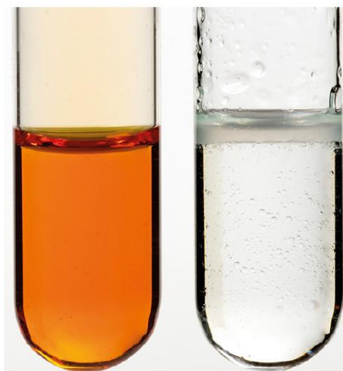
Figure: decolorization of bromine water by unsaturated compound
